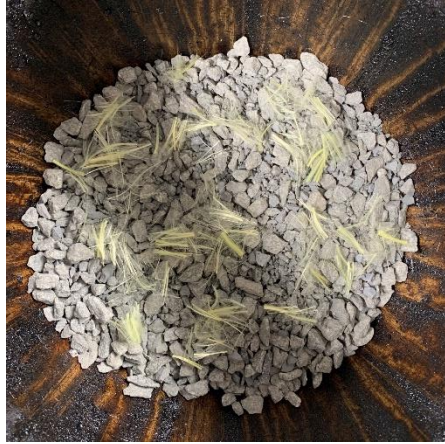
(a) Aggregate/Aramid layering
