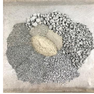
(b) Graded aggregate blend
